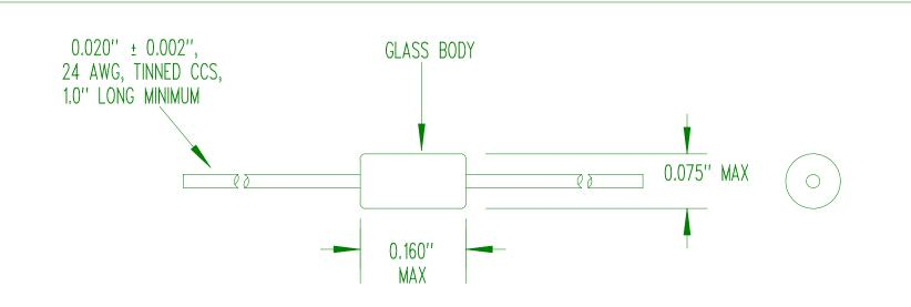
RESISTANCE @  $+25^{\circ}C = 30,000 \ \Omega \pm 1\%$  RESISTANCE RATIO  $(0/+50^{\circ}C) = 9.06$  NOMINAL RESISTANCE/TEMPERATURE CURVE = "J" TEMPERATURE COEFFICIENT @  $+25^{\circ}C = -4.4\%$  NOMINAL BETA " $\beta$ "  $(0\ TO\ +50^{\circ}C) = 3,892^{\circ}K$  NOMINAL (STILL AIR) THERMAL TIME CONSTANT =  $2\ mW/^{\circ}C$  NOMINAL (STILL AIR) THERMAL TIME CONSTANT =  $0.5\ SECONDS$  NOMINAL (STIRRED LIQUID) MAXIMUM OPERATING TEMPERATURE =  $+300^{\circ}C$
