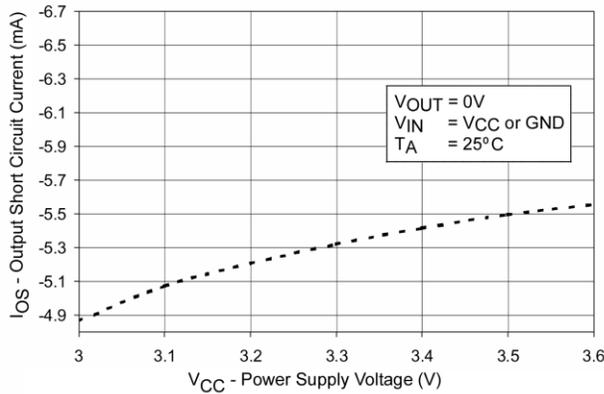
**Figure 7. Output Short Circuit Current vs. Power Supply Voltage**
