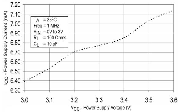
**Figure 12. Power Supply Current vs. Power Supply Voltage**
