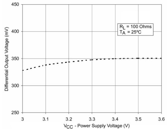
**Figure 8. Differential Output Voltage vs. Power Supply Voltage**
