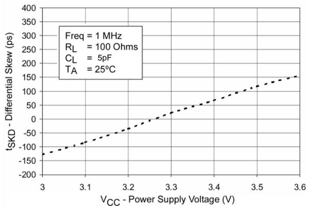
**Figure 16. Differential Pulse Skew ( $t_{PLH} - t_{PHL}$ ) vs. Power Supply Voltage**
