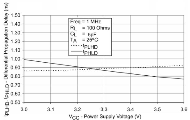
**Figure 14. Differential Propagation Delay vs. Power Supply**
