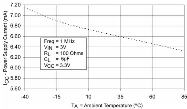
**Figure 13. Power Supply Current vs. Ambient Temperature**
