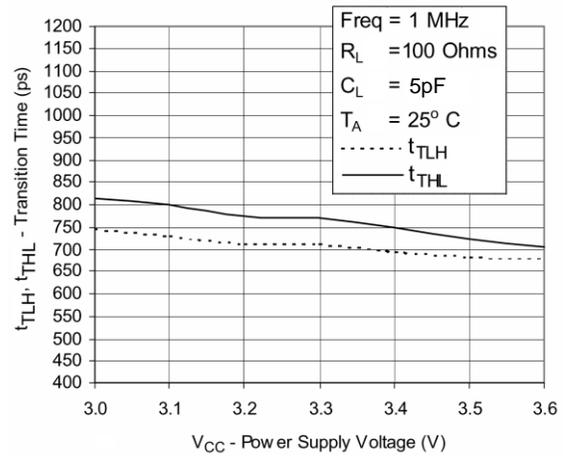
Figure 18. Transition Time vs. Power Supply Voltage
