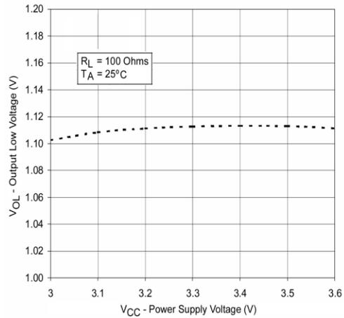
**Figure 6. Output Low Voltage vs. Power Supply Voltage**
