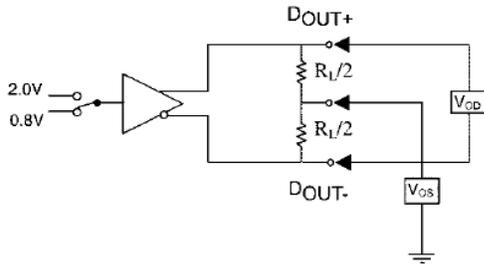
Figure 2. Differential Driver DC Test Circuit
