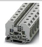
Thermoelectric voltage terminal block with bolt connection technology, cross section: 0.1 - 6 mm², AWG: 26 - 10, width: 16.3 mm, color: gray
