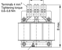
PE M4 / Tightening torque 1.2±0.1 Nm
