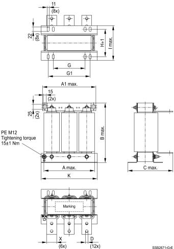
General tolerances according to ISO 2768-cL Dimensions in mm
