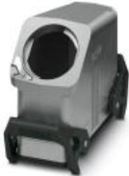
HEAVYCON EVO coupling housing, EMC version, without powder coating, with bayonet flange for EVO screw connection, B24, with double locking latch, height: 90 mm, without EVO screw connection.
