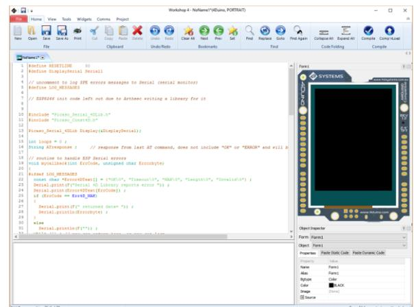
4DUINO Basic Graphics is designed primarily for use when no uSD card will be used with the display. Graphics primitives can be dragged and dropped onto the screen and the place in your code where the primitive is to be used can be located and the code pasted into the editor.
