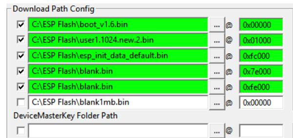
Again, the ESP-06 needs to be placed into Bootloader mode. To do this, simply press and hold the WiFi Flash button on the 4Duino, and press the WiFi Reset button for a second and then release the Reset button. Keep holding the WiFi Flash button. A second or so later, you can release the WiFi Flash button. The ESP-06 should now be in Bootloader mode.
