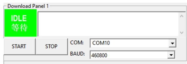
Before anything is programmed, the ESP8266 module needs to be wiped blank. It is always best to do this before programming in any new firmware, as residual data can be left which can cause unexpected results.
