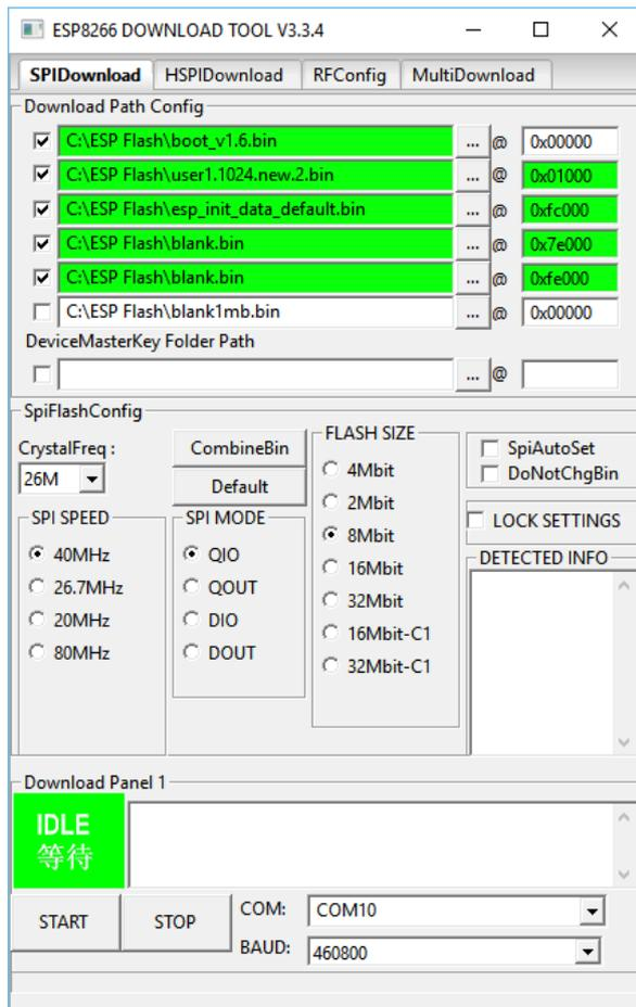
It will be noticed there are 6 different files preloaded into the Download Path Config boxes. These need to be changed to the location where the files were extracted.
