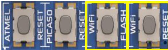
Press the Start Button, to start the programming of the ESP-06 module.
