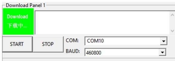
Then the application will load and the ESP8266 is wiped blank. It will complete when the progress bar goes to the very right hand side.
