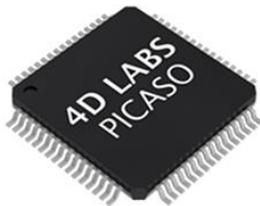
The PICASO processor is a custom graphics processor, where all functionality including the high level commands are built into the chip.
