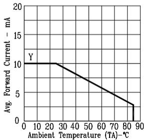
Fig8. MAX. AVERAGE FORWARD CURRENT VS. AMBIENT TEMPERATURE.
