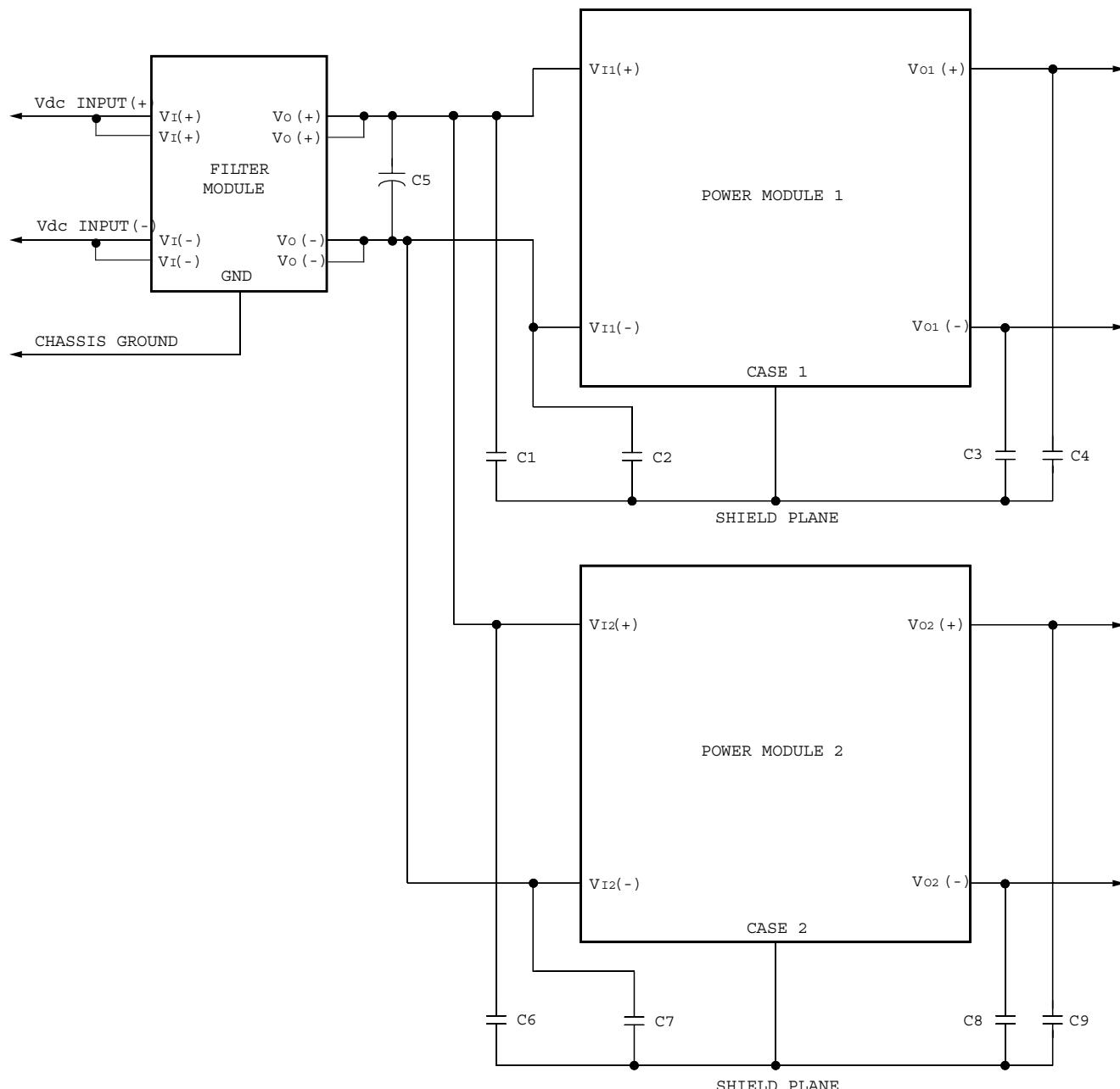
Note: C1 through C4 and C6 through C9 can be 0.01  $\mu$ F to 0.1  $\mu$ F. Select the voltage rating to meet input-to-output isolation requirements.
