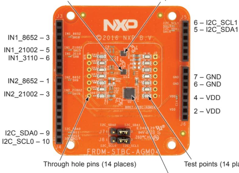
FXAS21002C 3-axis digital angular rate gyroscope
