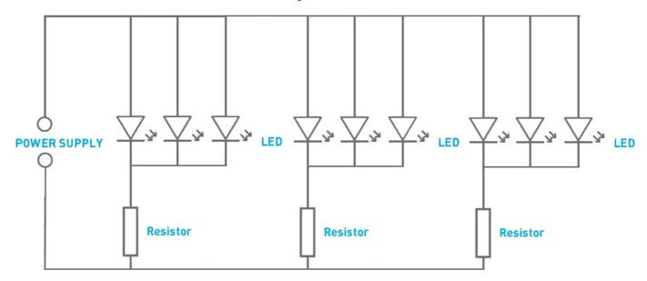
The circuit diagram for the 5V LED Desk Lamp is shown above. It is a very simple circuit. The board contains nine LEDs, these are grouped in to threes, with each group of three sharing a current limit resistor.
