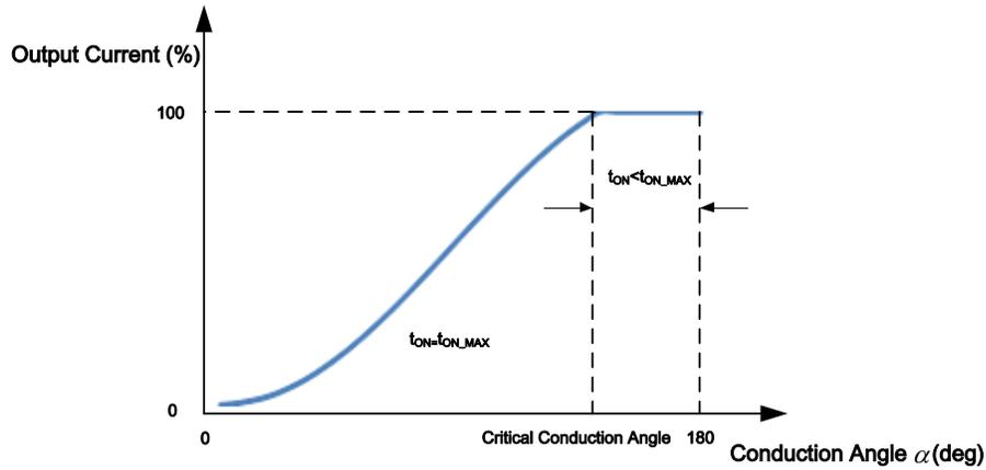
Figure.2 Dimming Curve
