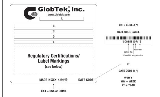
A=Medical/ITE/Household use Power Supply B=P/N: (料号) RR9LX750T00-IMR6B C=Model (型号) GTM96300-3648-R3A D=Input (输入) 100-240V~, 50-60 Hz, 1.0A
