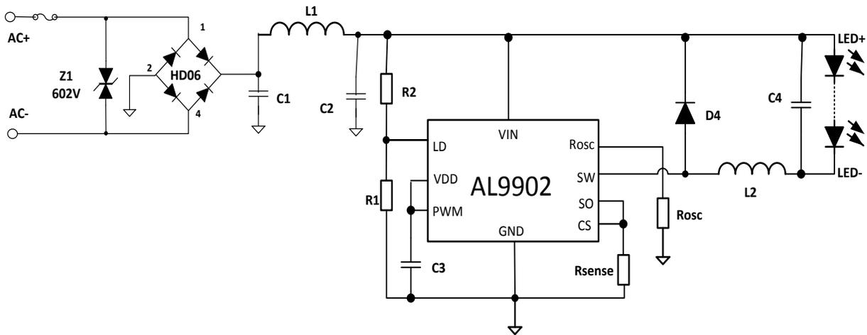
**Figure 2 Typical Application Circuit with Simple PFC**
