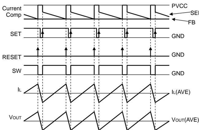
Fig.28 PWM switching timing chart
