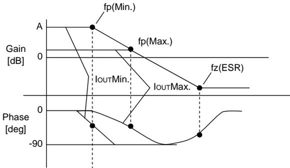
Fig.36 Open loop gain characteristics
