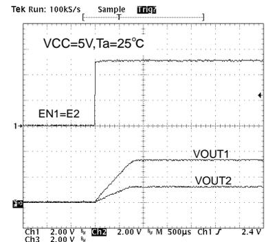
Fig.14 Soft start waveform (I<sub>o</sub>=0mA)
