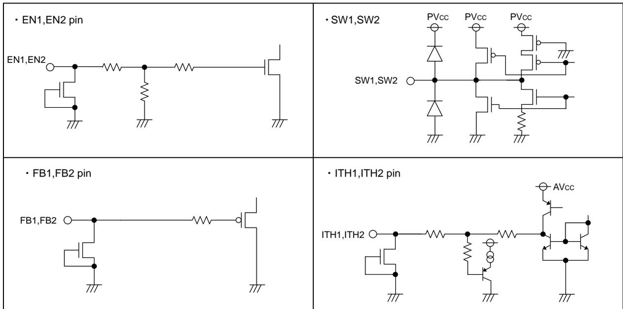
Fig.41 I/O equivalence circuit
