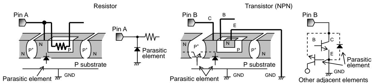
Fig.42 Simplified structure of monolithic IC
