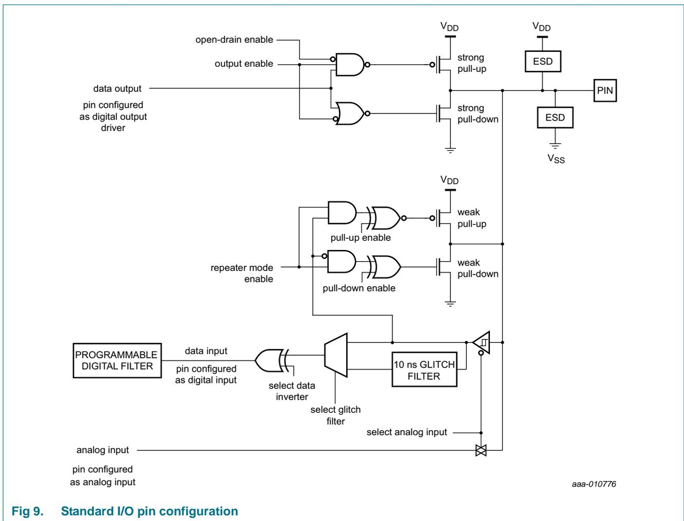
Fig 9. Standard I/O pin configuration
