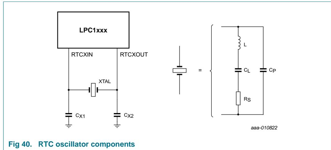
Fig 40. RTC oscillator components
