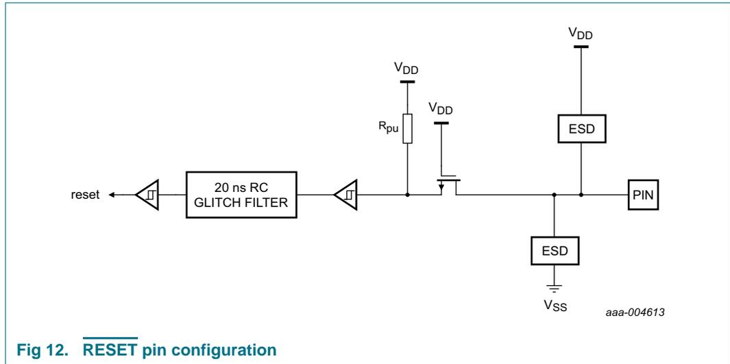
Fig 12. RESET pin configuration
