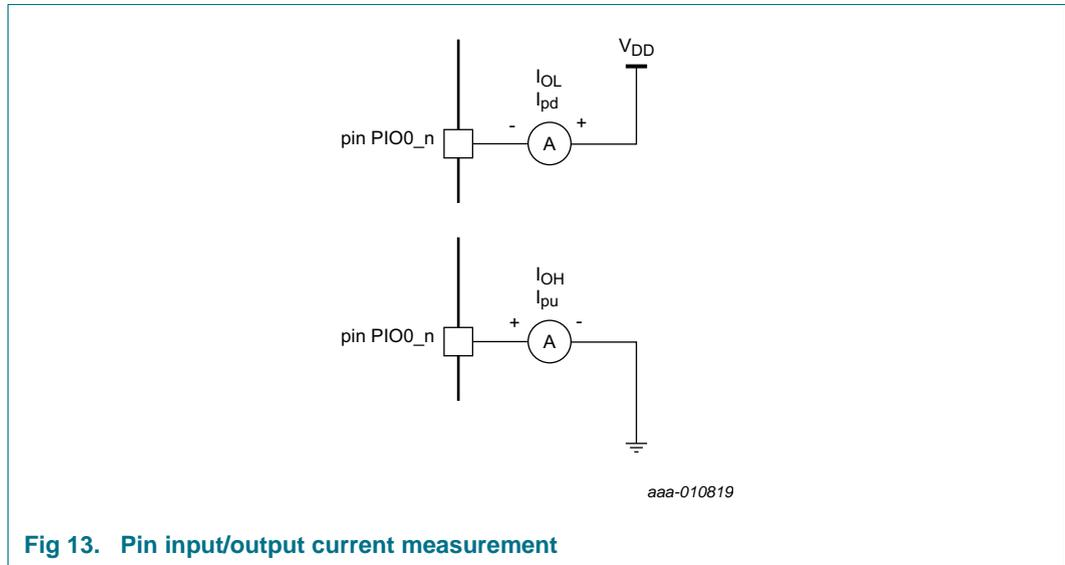
**Fig 13. Pin input/output current measurement**
