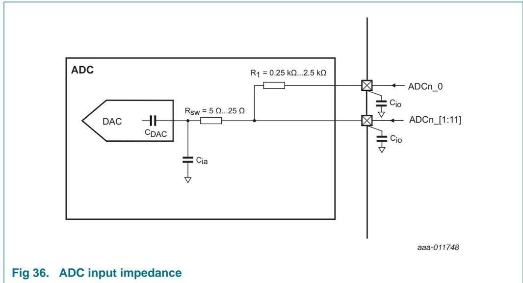
Fig 36. ADC input impedance
