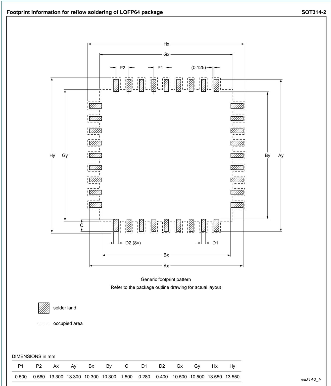
**Fig 46. Reflow soldering for the LQFP64 package**
