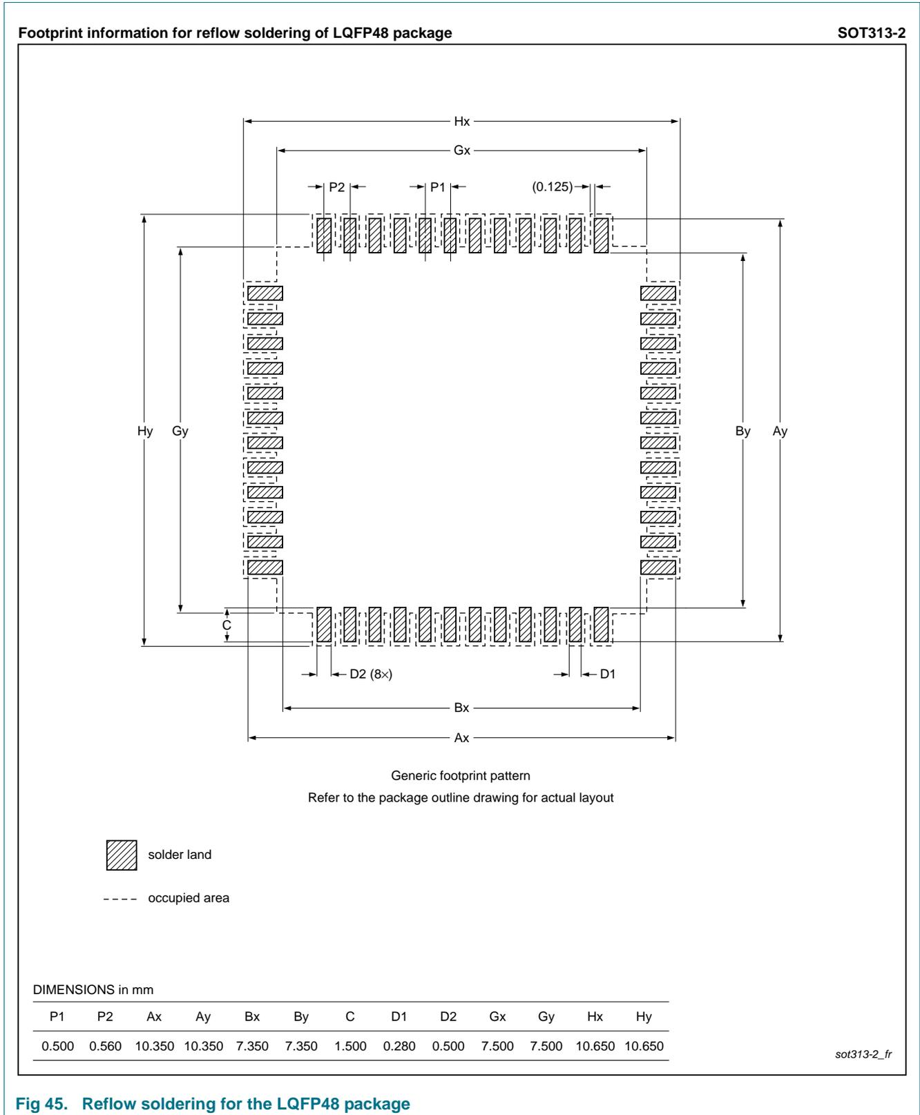
Fig 45. Reflow soldering for the LQFP48 package
