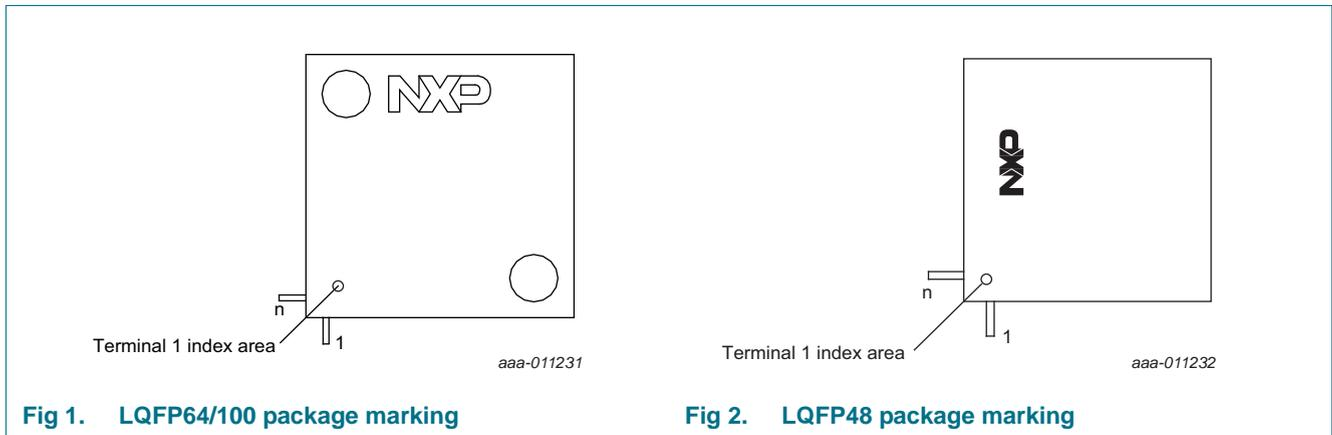
Fig 1. LQFP64/100 package marking
