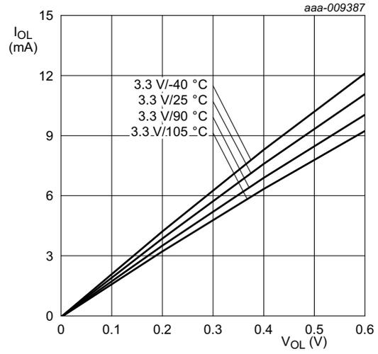
Conditions:  $V_{DD} = 3.3$  V; standard port pins and high-drive pins PIO0\_7 and PIO1\_31.
