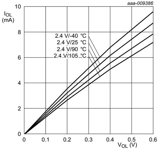
Conditions:  $V_{DD} = 2.4$  V; standard port pins and high-drive pins PIO0\_7 and PIO1\_31.
