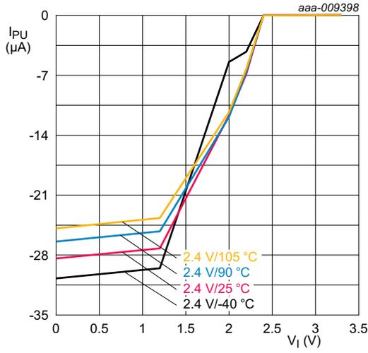
Conditions:  $V_{DD} = 2.4$  V; standard port pins.
