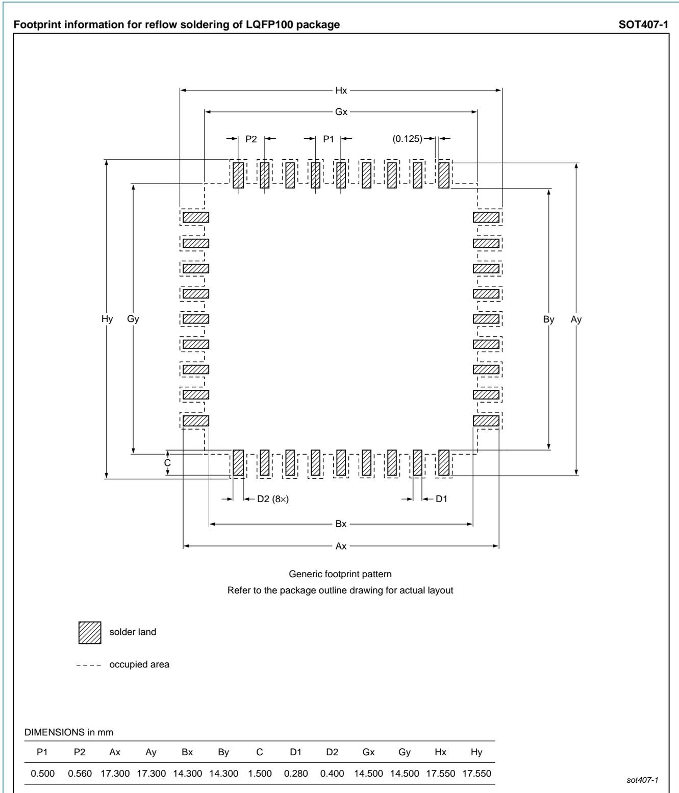
**Fig 47. Reflow soldering for the LQFP100 package**
