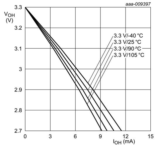
Conditions:  $V_{DD} = 3.3$  V; standard port pins.
