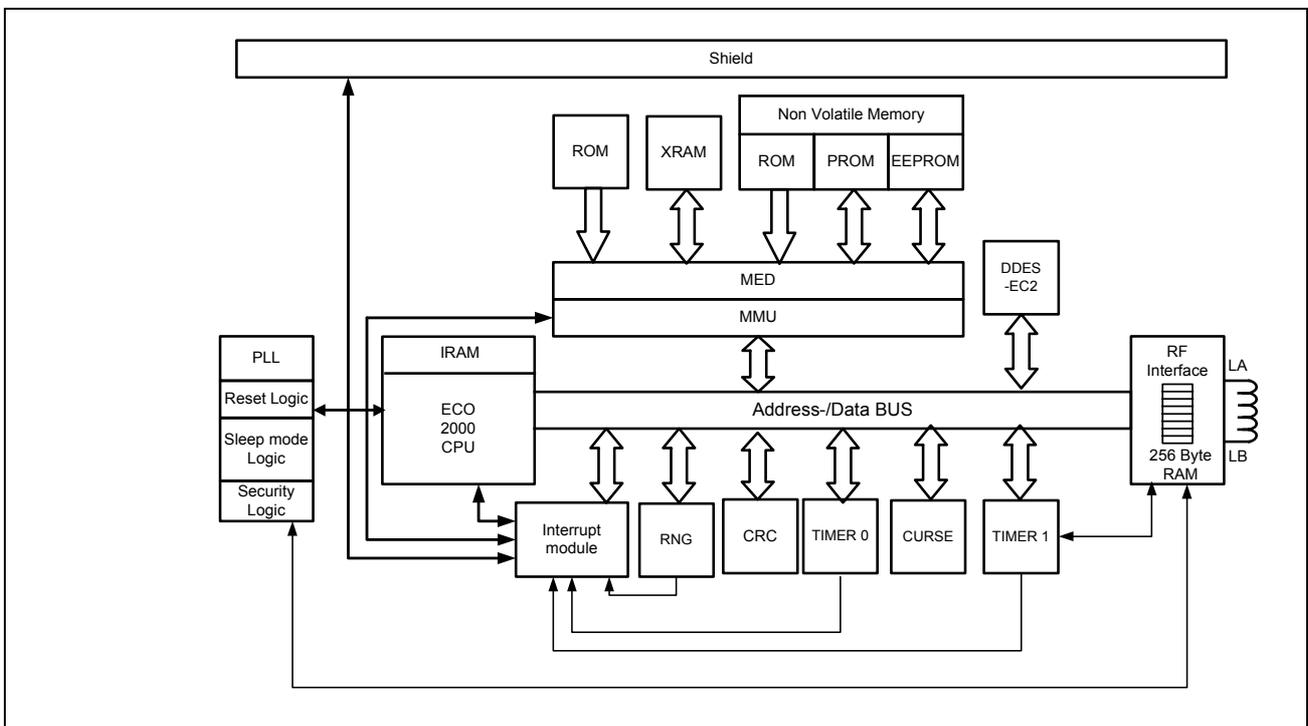
**Figure 2: Block Diagram of SLE 66CL81P**
