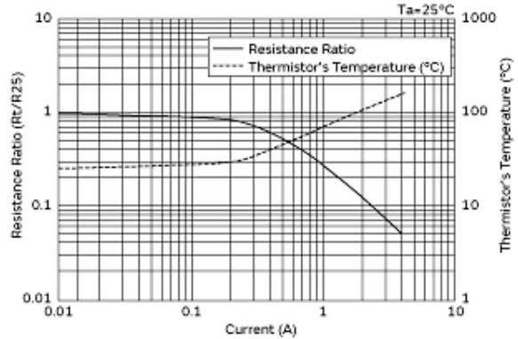
Current-R ratio( $R_t/R_{25}$ ), Current-Temperature Characteristics
