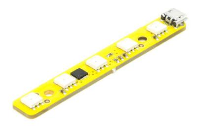
The Rainbow module has five shiny bright full-colour LEDs. It's ideal for using as a readout of sensor values, mood light, or health bar indicator for a game.
