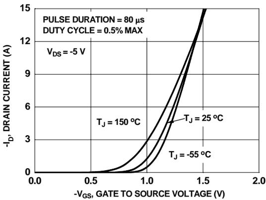
**Figure 5. Transfer Characteristics**
