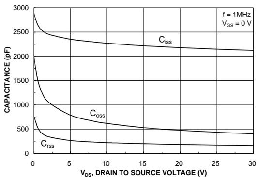
Figure 8. Capacitance Characteristics.
