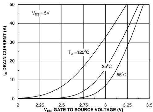
Figure 5. Transfer Characteristics.
