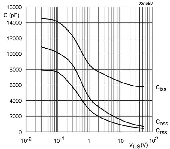
$$V_{GS} = 0\text{V}; f = 1\text{MHz}$$
