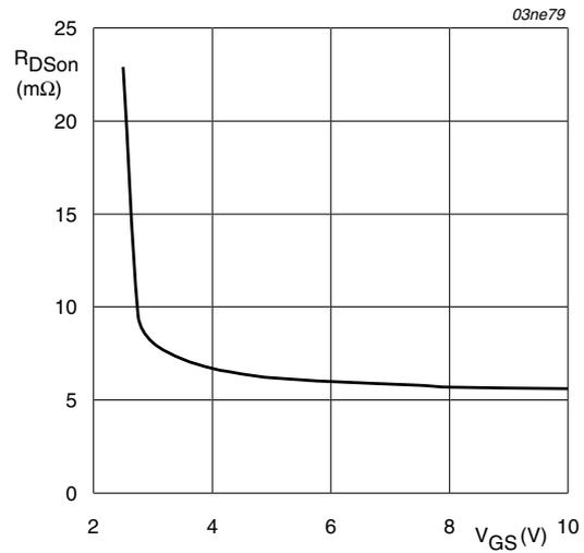
$T_j = 25^\circ\text{C}; I_D = 50\text{A}$
