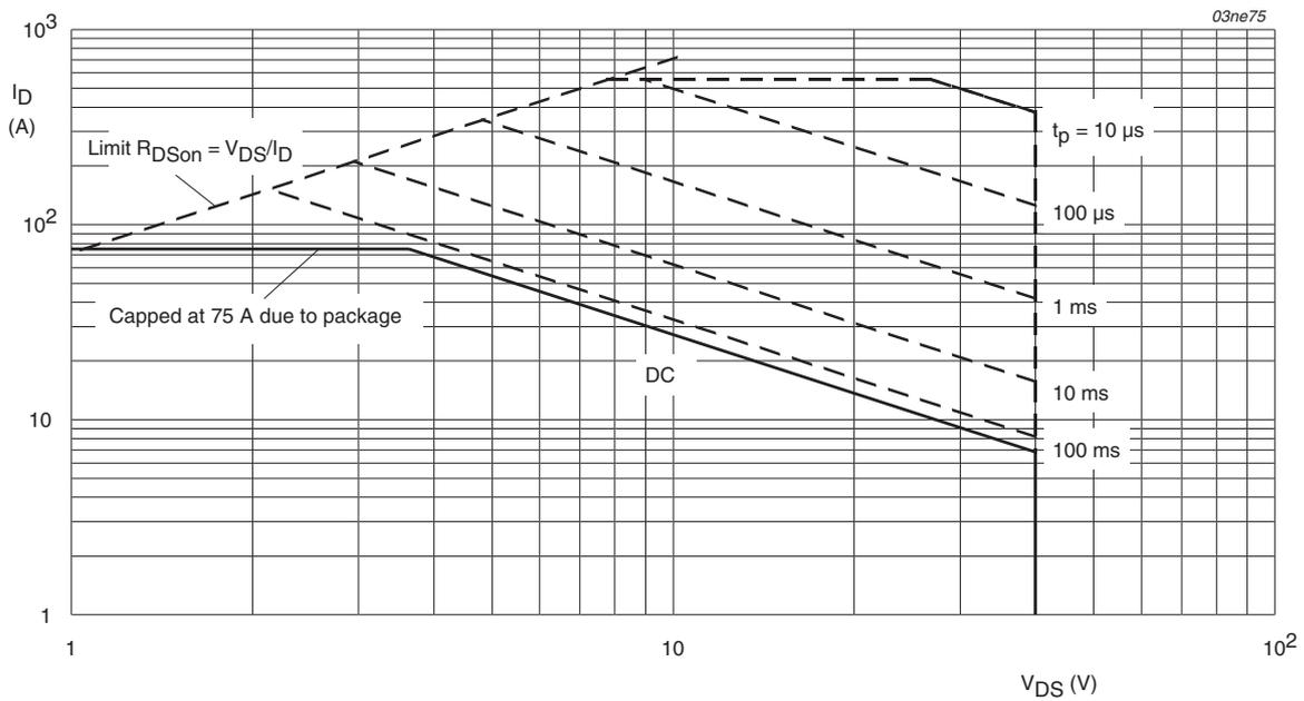
$$T_{mb} = 25^\circ C; I_{DM} \text{ is single pulse}$$
