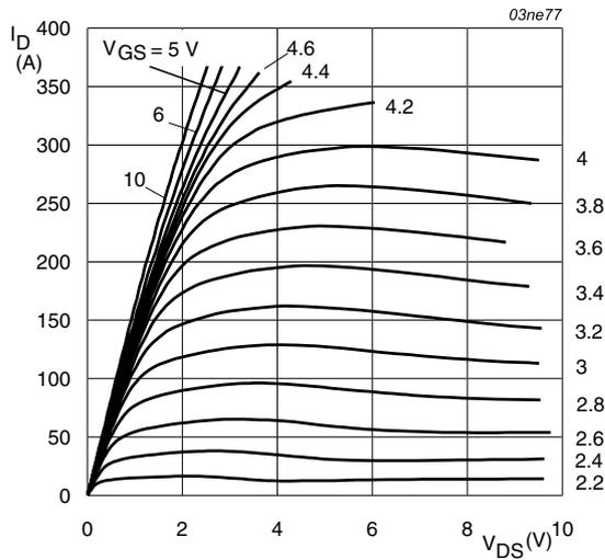
$T_j = 25^\circ\text{C}; t_p = 300\mu\text{s}$
