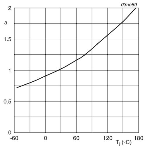
$$a = \frac{R_{DSon}}{R_{DSon(25^\circ\text{C})}}$$
