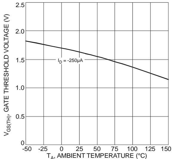
Figure 14 Gate Threshold Variation vs. Ambient Temperature
