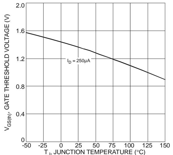
Figure 6 Gate Threshold Variation vs. Ambient Temperature
