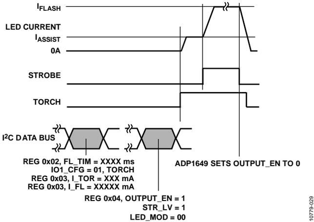
Figure 29. Enabling Flash Mode from External Torch Mode
