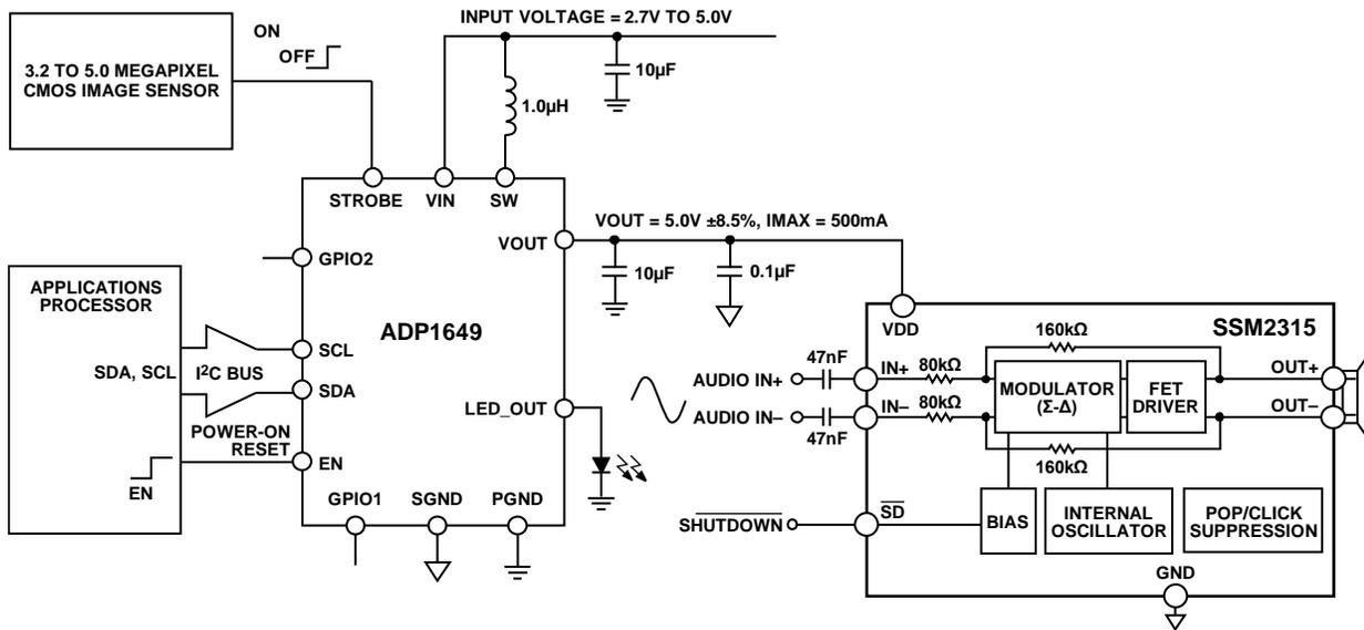
Figure 38. Voltage Regulation Mode: Class-D Audio Application
