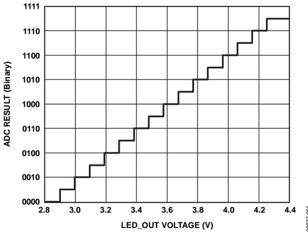
Figure 18. ADC LED  $V_f$  Mode Transfer Characteristic
