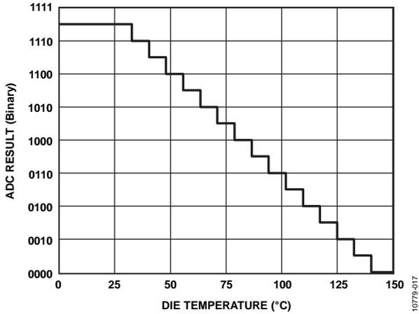
Figure 17. ADC Die Temperature Mode Transfer Characteristic
