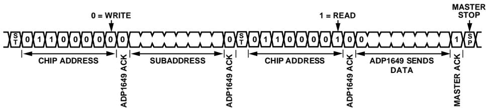
Figure 40. I<sup>2</sup>C Single Register Read Sequence
