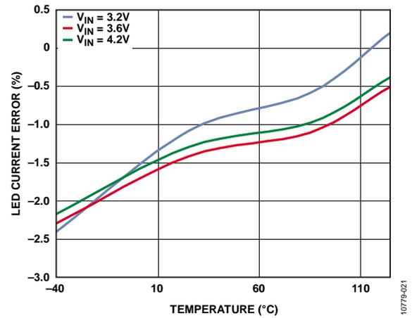
Figure 21. LED Current Error vs. Temperature,  $I_{LED} = 800$  mA
