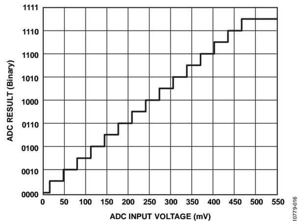
Figure 16. ADC External Voltage Mode Transfer Characteristic
