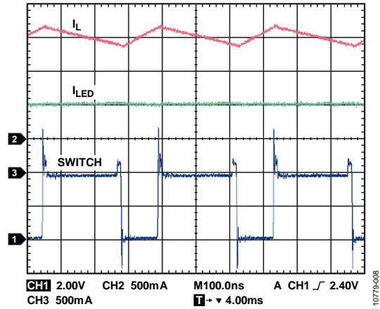
Figure 8. Switching Waveforms, Flash Mode,  $I_{LED} = 1000\text{ mA}$
