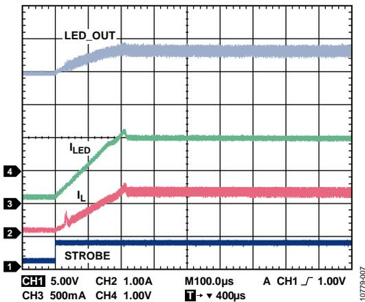
Figure 7. 100 mA Torch to 1000 mA Flash Transition
