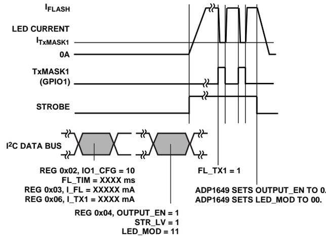
Figure 30. TxMASK1 Operation During Flash (Level Sensitive) Mode
