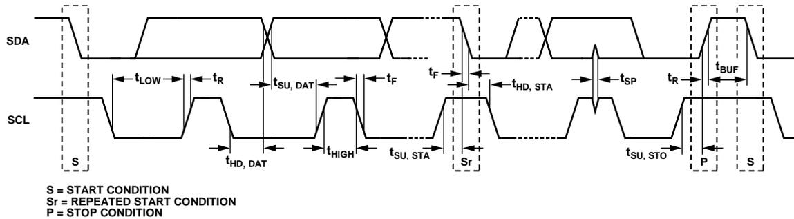
Figure 3. I<sup>2</sup>C-Compatible Interface Timing Diagram
