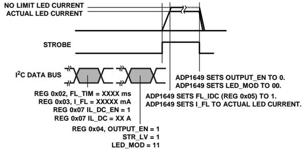
Figure 32. DC Current-Limit Operation in a Low Battery, High LED V<sub>F</sub> Case
