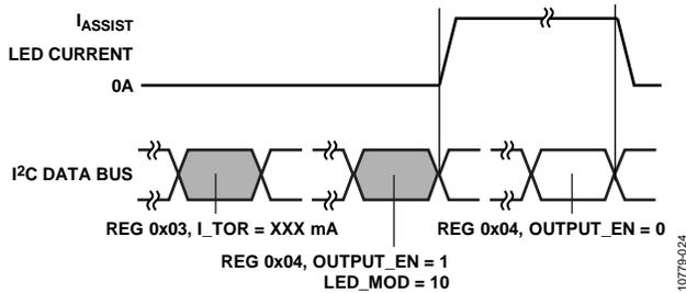
Figure 24. Enabling and Disabling Assist Light Mode
