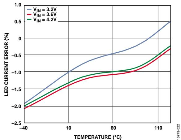
Figure 22. LED Current Error vs. Temperature,  $I_{LED} = 1000$  mA
