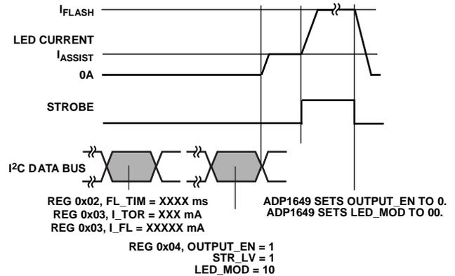
Figure 27. Enabling Assist to Flash (Level Sensitive) Mode
