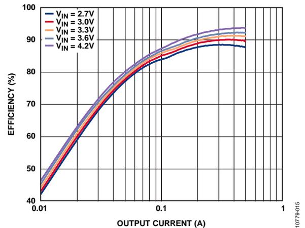
Figure 15. Voltage Regulation Mode Efficiency vs. Load Current
