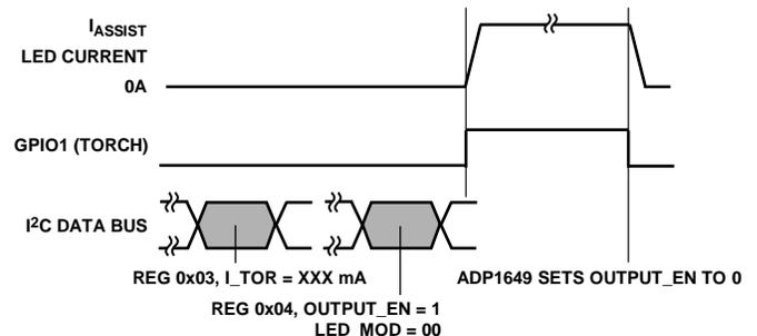
Figure 28. Enabling External Torch Mode Using GPIO1
