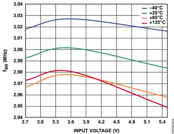
Figure 12. Switching Frequency vs. Supply Voltage (3 MHz Mode)
