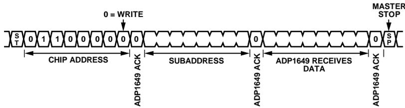
Figure 39. I<sup>2</sup>C Single Register Write Sequence
