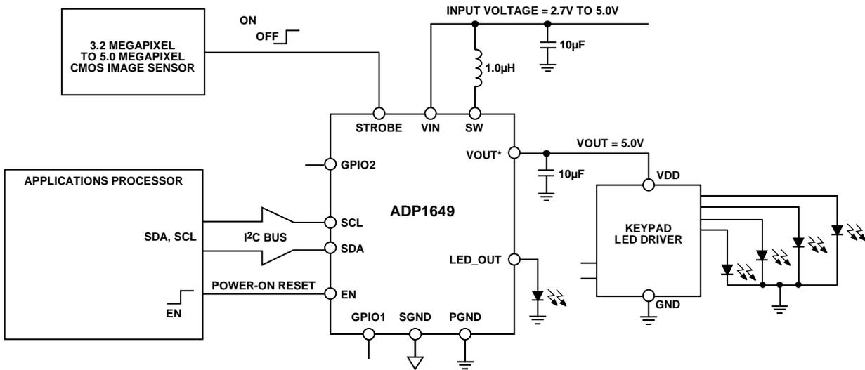
\*THE VOUT PIN IS CONNECTED TO THE SW NODE WHEN THE ADP1649 IS NOT ENABLED. VOUT SHOULD NOT BE CONNECTED DIRECTLY TO A POSITIVE EXTERNAL VOLTAGE SOURCE BECAUSE THIS CAUSES CURRENT TO FLOW FROM VOUT TO THE BATTERY.
