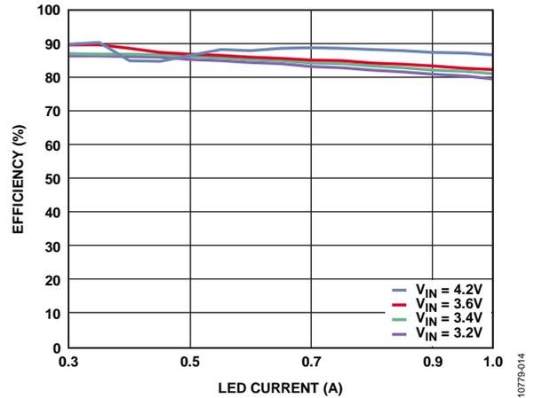
Figure 14. Flash Mode Efficiency vs. LED Current
