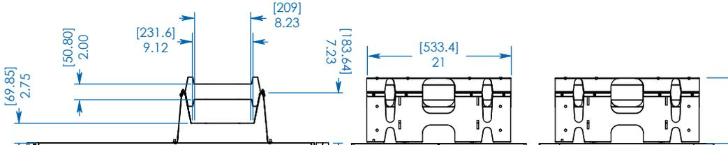
OPTIONAL SRCABLETRAY AND SRCABLETRAYEXP CABLE MANAGEMENT ACCESSORIES SHOWN (MOUNTING POSITION ADJUSTS TO ACCOMMODATE A WIDE RANGE OF APPLICATIONS)
