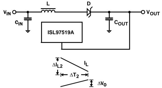
FIGURE 13. BOOST CONVERTER - CYCLE 2, POWER SWITCH OPEN
