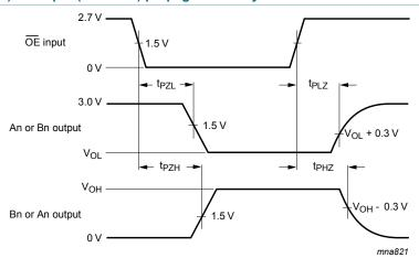
$V_{\text{OL}}$  and  $V_{\text{OH}}$  are typical voltage output levels that occur with the output load.
