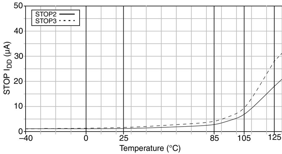
Figure 3-7. Typical Stop I<sub>DD</sub> vs. Temperature (V<sub>DD</sub> = 5V)
