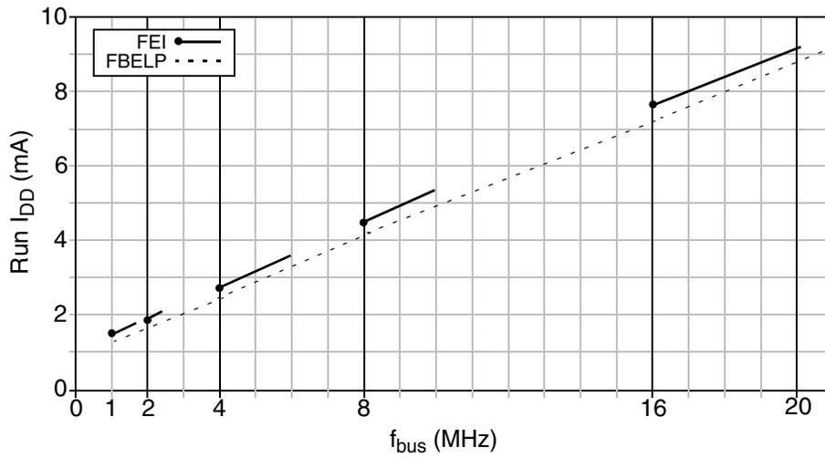
Figure 3-5. Typical Run I<sub>DD</sub> vs. Bus Frequency (V<sub>DD</sub> = 5V)
