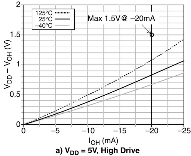
Figure 3-3. Typical  $V_{DD} - V_{OH}$  vs  $I_{OH}$ , High Drive Strength
