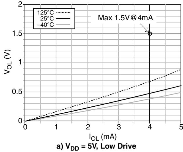
Figure 3-2. Typical  $V_{OL}$  vs  $I_{OL}$ , Low Drive Strength
