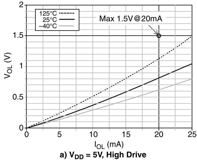
Figure 3-1. Typical  $V_{OL}$  vs  $I_{OL}$ , High Drive Strength
