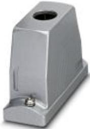
HEAVYCON ADVANCE standard powder-coated sleeve housing B16, with screw locking, height 100 mm, with 1x M25 thread, straight cable outlet
