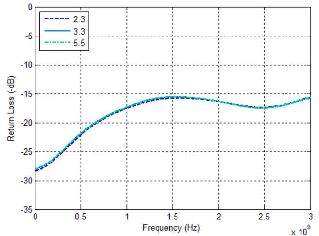
**Figure 9. RFC Port Return Loss vs. Temp (RF2 Active)**
