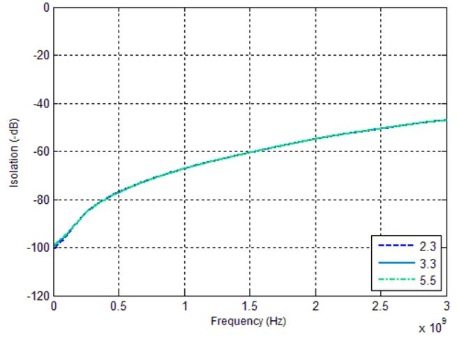
**Figure 17. Isolation vs. Temp (RFC-RFX)**
