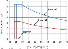
Figure 1. Typical Input Characteristic at Room Temperature.
