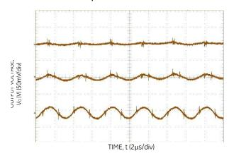
Figure 9. Typical Output Ripple and Noise at Room Temperature  $I_0$  =  $I_{0,max}$  and and  $C_{OMin}$ .
