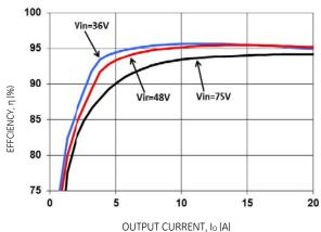
Figure 2. Typical Converter Efficiency  $\overline{\text{Vs.}}$  Output current at Room Temperature.
