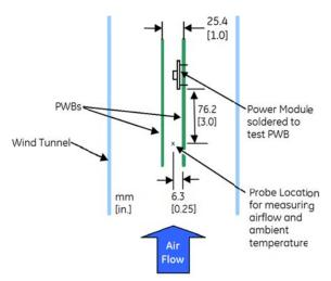
Heat-dissipating components are mounted on the top side of the module. Heat is removed by conduction, convection and radiation to the surrounding environment. Proper cooling can be verified by measuring the thermal reference temperature (TH<sub>x</sub>). Peak temperature (TH<sub>x</sub>) occurs at the position indicated in Figure 18 and 19. For reliable operation this temperature should not exceed the listed temperature threshold.
