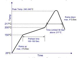
Figure 23. Recommended linear reflow profile using Sn/Ag/Cu solder.
