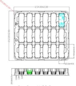
Open Frame Module Tray Figure 25. EBVW020 Packaging Tray
