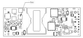
Figure 18. Location of the thermal reference temperature TH<sub>1</sub>. Do not exceed 113 °C.
