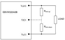
Figure 17. Circuit Configuration to Trim Output Voltage.
