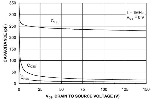
Figure 8. Capacitance Characteristics.
