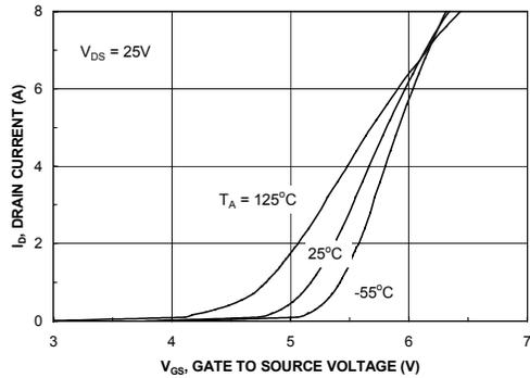
Figure 5. Transfer Characteristics.
