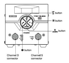
The front panel of the HAKKO FM-203 has four controls.
