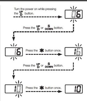
The channel D setting is completed as shown in the preceding diagram. Repeatedly pressing the button moves to the channel S setting. (The process is the same as that for channel D.)
