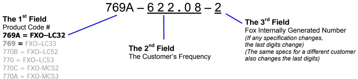
This example, **FXO-LC325R-622.08** = LVDS Output, Ceramic, 3.2 x 2.5mm Package, 2.5V, ±50 PPM Stability, -40 to +85°C Temperature Range, at 622.08 MHz
