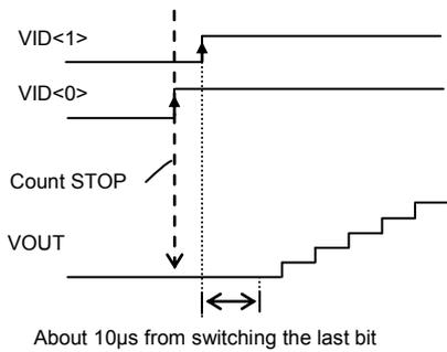
Fig.26 Timing chart of setting the output voltage
