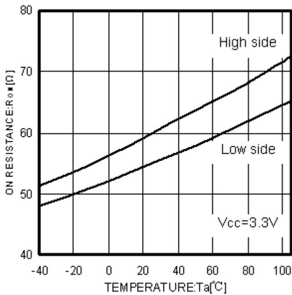
Fig.10 Ta-R<sub>ON</sub>, R<sub>ONP</sub>
