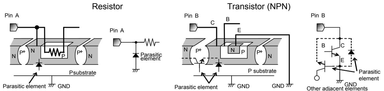
Fig.41 Simplified structure of monoristic IC
