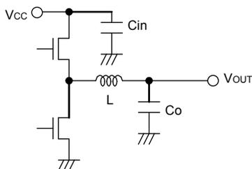
Fig.33 Input capacitor
