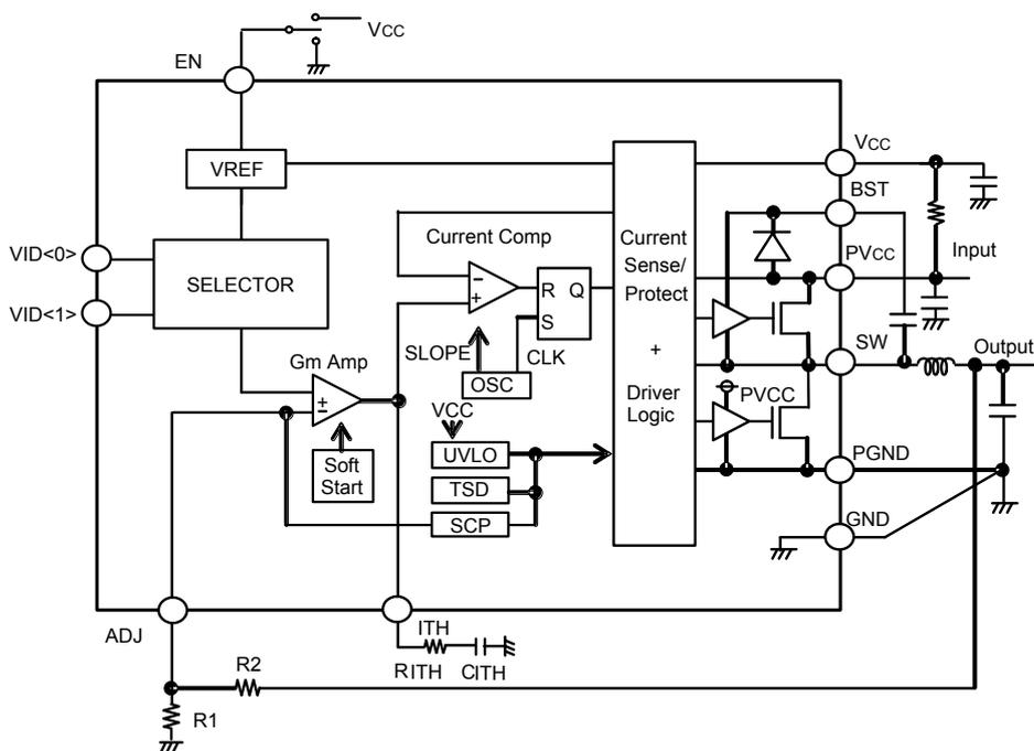
Fig.3 Block Diagram
