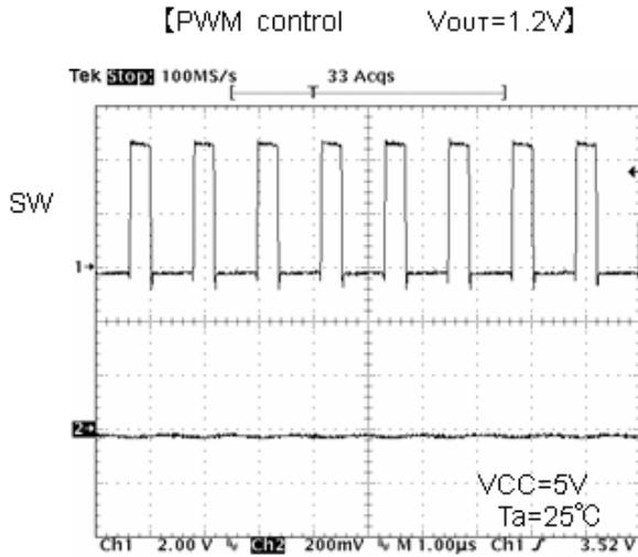
Fig.16 SW waveform  $I_o=4A$
