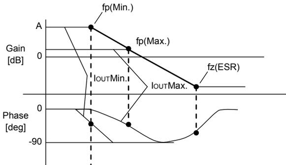
Fig.34 Open loop gain characteristics
