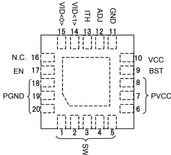
Fig.2 Pin configuration
