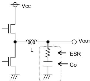
Fig.32 Output capacitor
