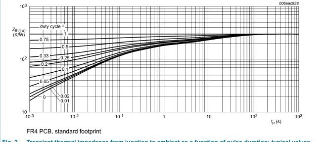
Transient thermal impedance from junction to ambient as a function of pulse duration; typical values Fig. 2.
