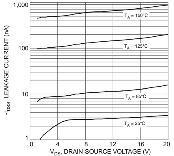
Fig. 20 Typical Leakage Current vs. Drain-Source Voltage
