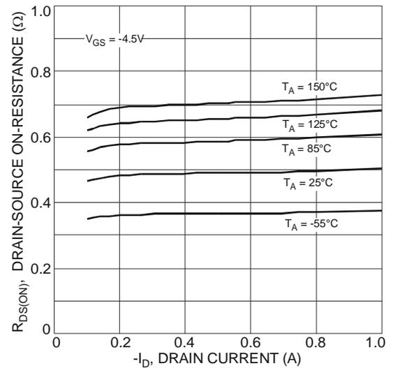
Fig. 14 Typical On-Resistance vs. Drain Current and Temperature
