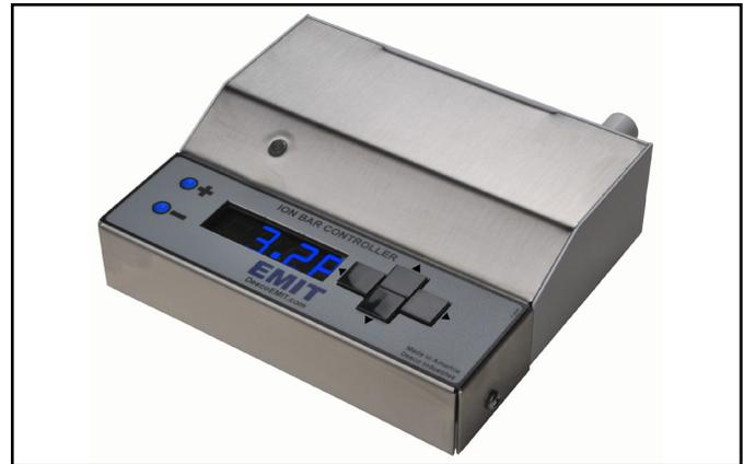
Figure 6. EMIT 50855 Controller with Digital Adjustment
