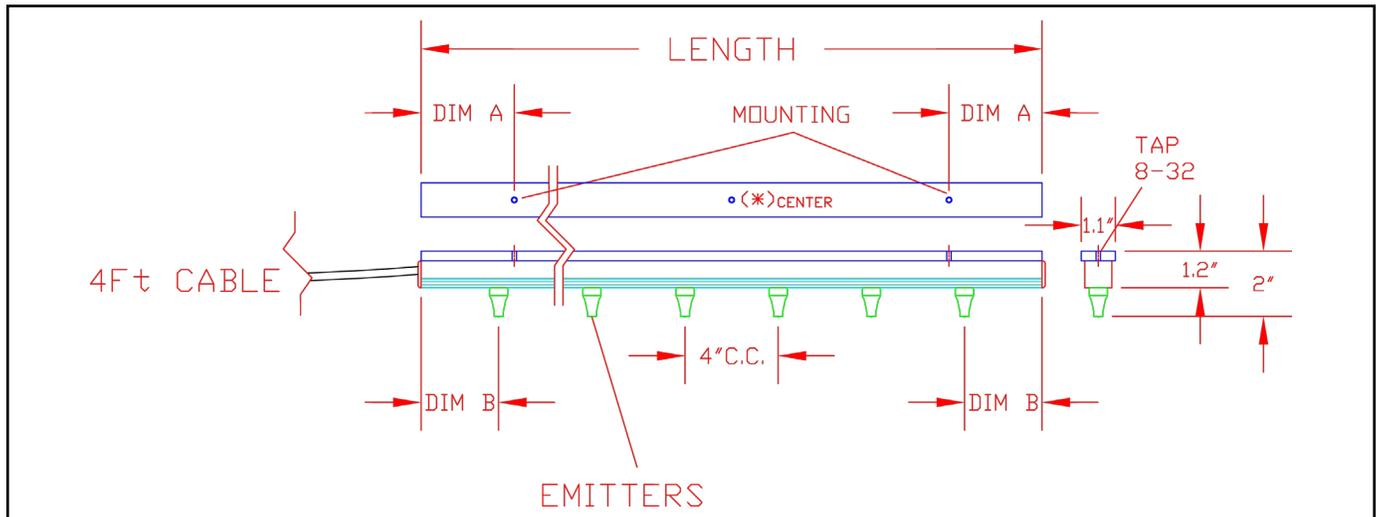
Figure 3. EMIT Non-Air Assisted Ion Bar dimensions
