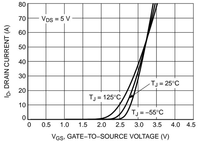
Figure 2. Transfer Characteristics
