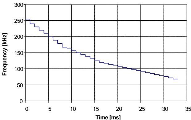
Figure 9 Switching frequency during softstart when  $R_{FMIN}=22k\Omega$
