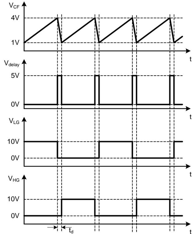
Figure 4 Oscillator waveforms
