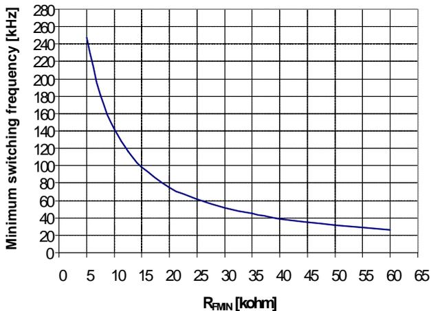
Figure 5  $F_{MIN}$  versus  $R_{FMIN}$
