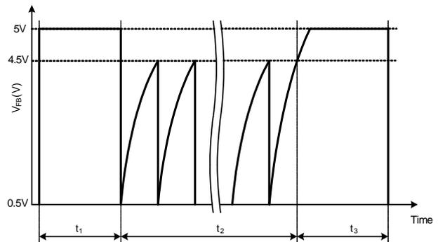
Figure 12 FB voltage waveform during over load protection
