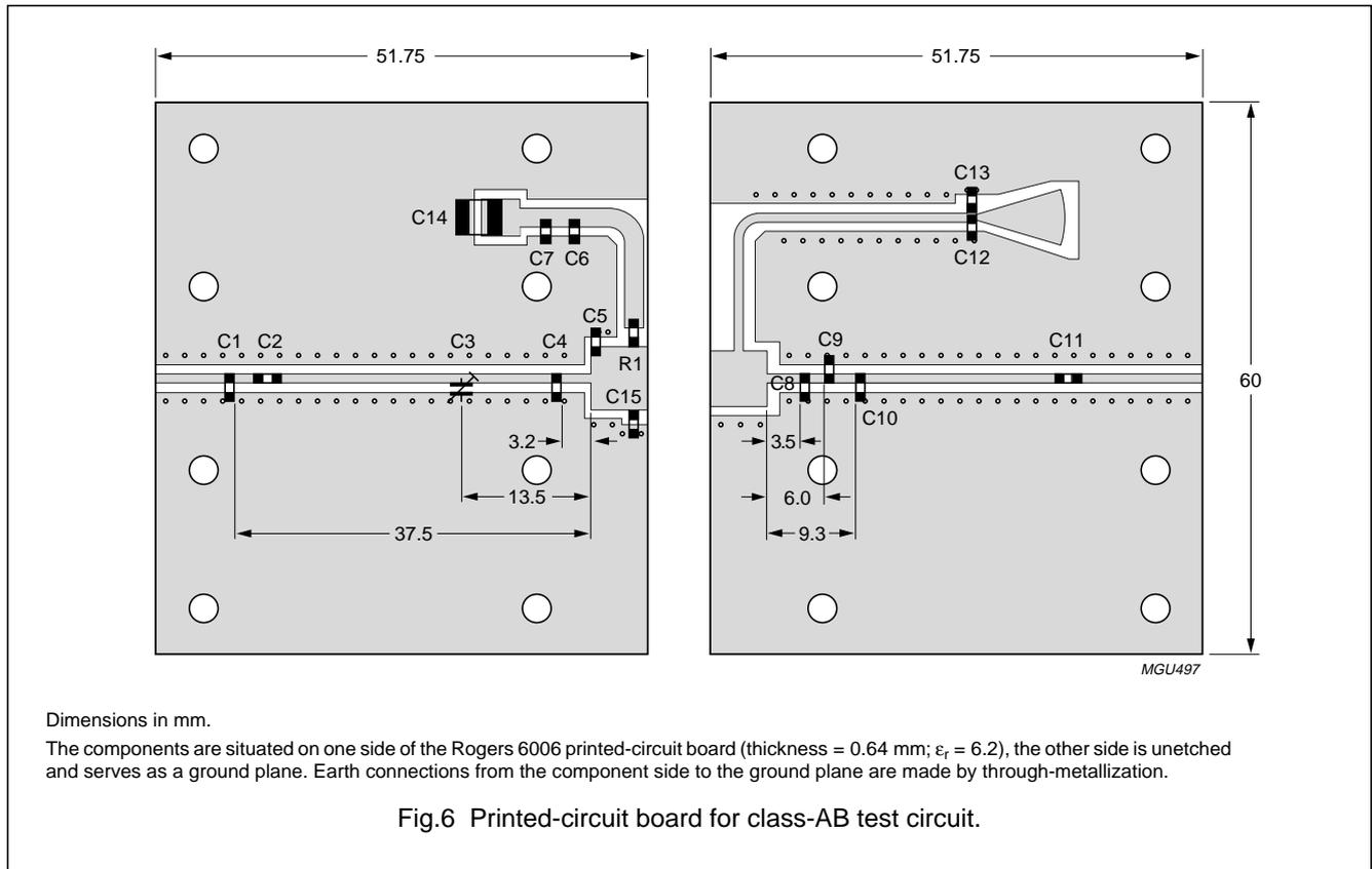
Fig.6 Printed-circuit board for class-AB test circuit.
