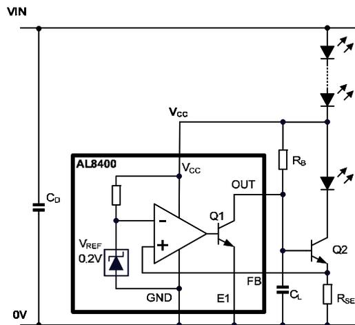
**Figure 11 High Voltage Operation Tapping V<sub>CC</sub> from the LED String**
