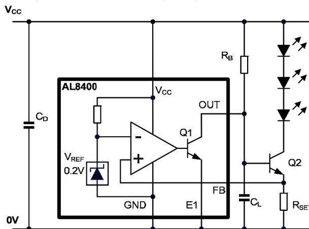
**Figure 2 Application Circuit Using Bipolar Transistor**
