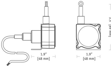
The SP2 String Pot from Celesco is a compact, economical and water resistant device that utilizes a flexible cable, a spring-loaded spool and a potentiometer to detect and measure linear position.
