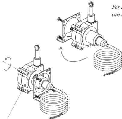
For added flexibility, mounting bracket can easily be switched to the opposite side.
