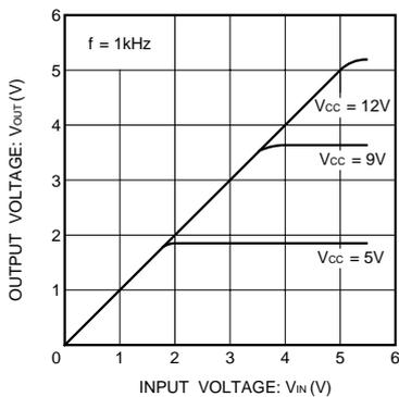
Fig. 2 V<sub>IN</sub> vs. V<sub>OUT</sub> characteristics (f = 1kHz)
