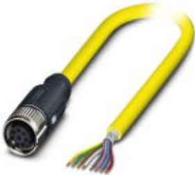
Sensor/Actuator cable, 8-position, PVC, yellow, shielded, Socket straight M12 SPEEDCON, A - standard, on free cable end, Cable length: 15 m
