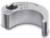
Nut for assembling sensor/actuator cables with M12 connector and M12 connectors for assembly, with a knurl diameter of 15 mm, for 4 mm hexagonal drive
