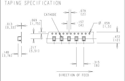
TOLERANCE: .004 UNLESS OTHERWISE SPECIFIED MILLIMETER DIMENSIONS SHOWN FOR REFERENCE ONLY
