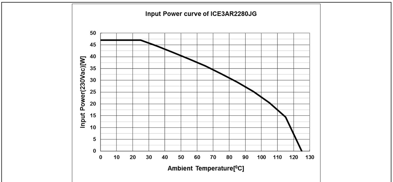
Figure 41 Input power curve  $V_{IN}=230 V_{AC}$ ;  $P_{in}=f(T_a)$
