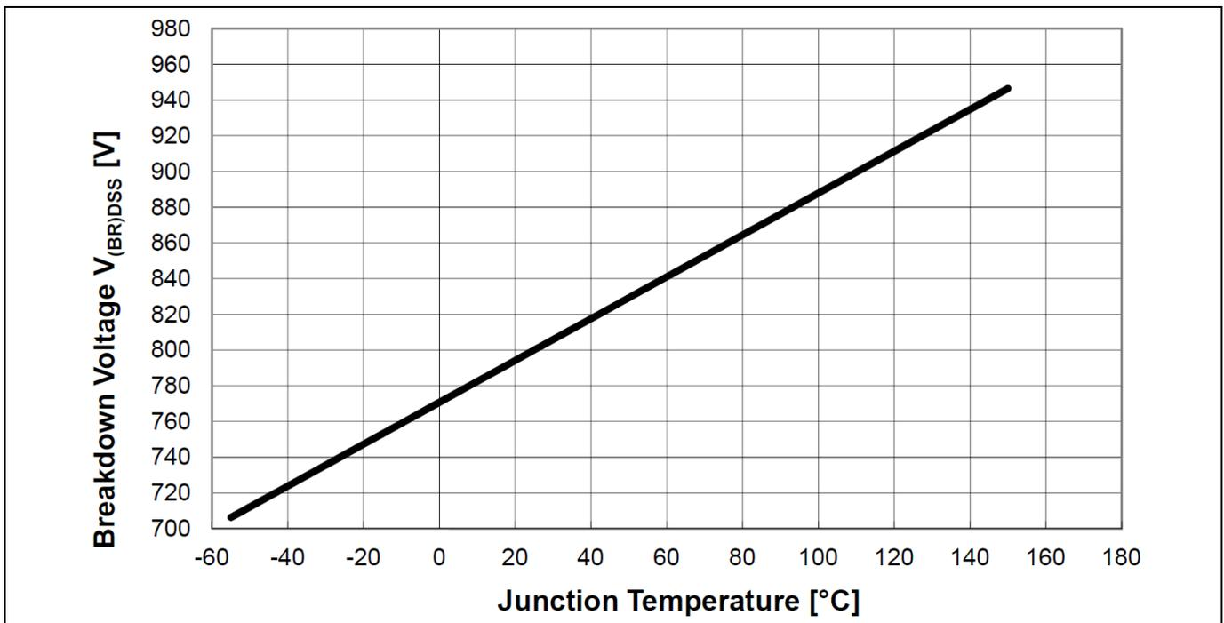
Figure 39 Drain-source breakdown voltage;  $V_{BR(DSS)}=f(T_j)$ ,  $I_D=0.25mA$
