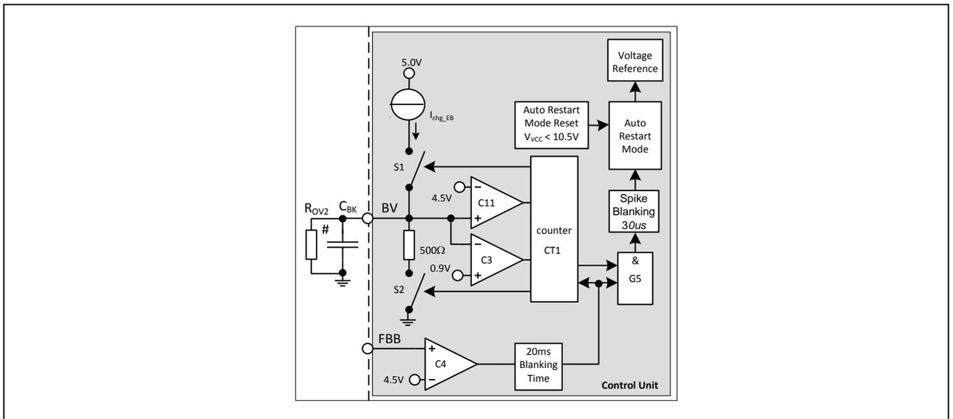
**Figure 33 Over load, open loop protection**
