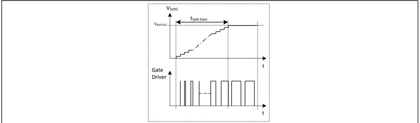
**Figure 13 Gate drive signal under Soft-Start Phase**
