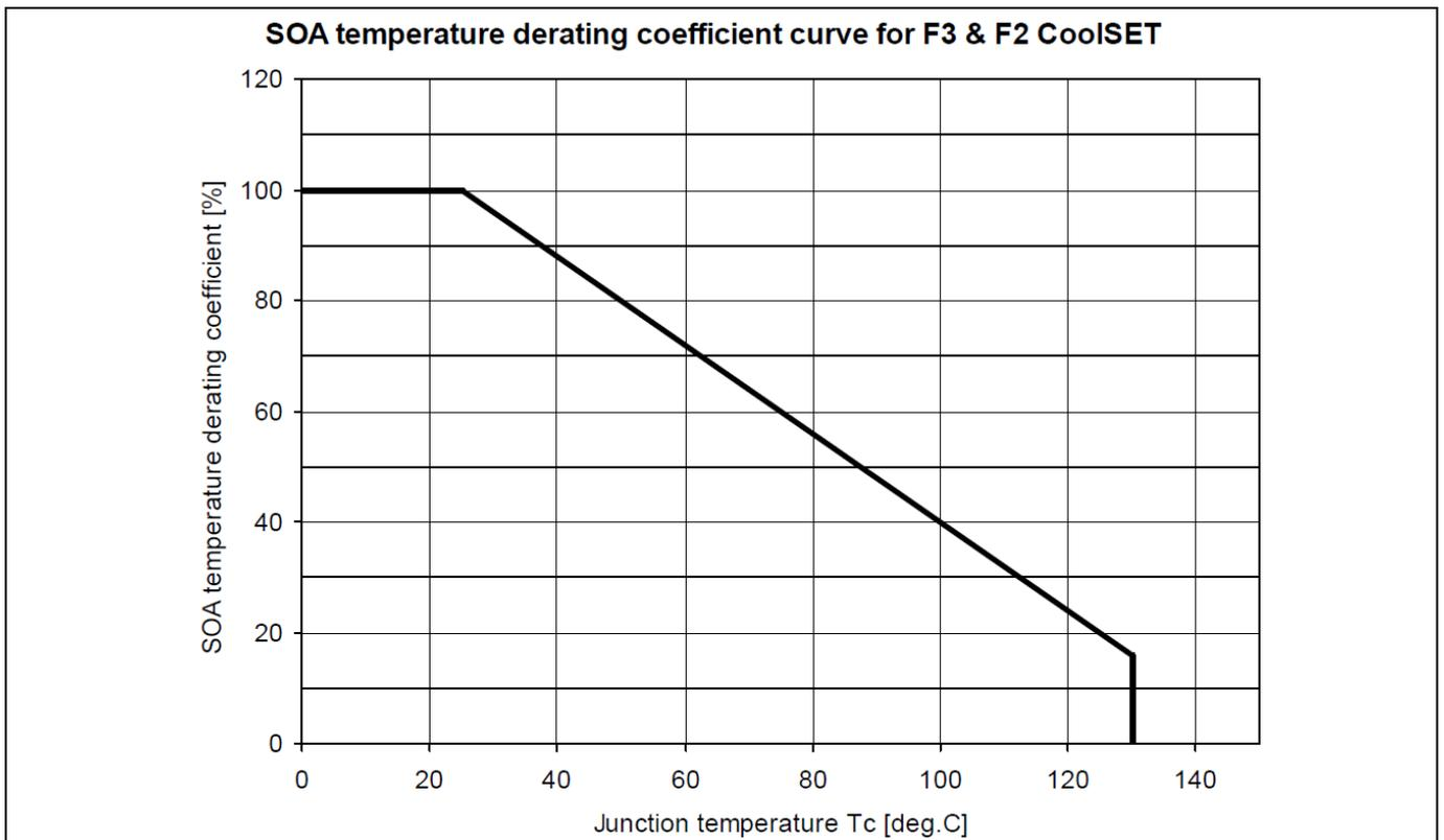
Figure 37 SOA temperature derating coefficient curve
