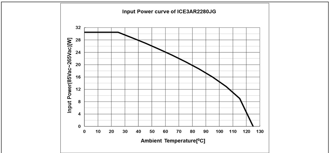
Figure 40 Input power curve  $V_{IN}=85 \sim 265 V_{AC}$ ;  $P_{in}=f(T_a)$
