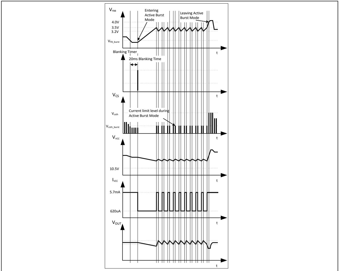
Figure 27 Signals in Active Burst Mode
