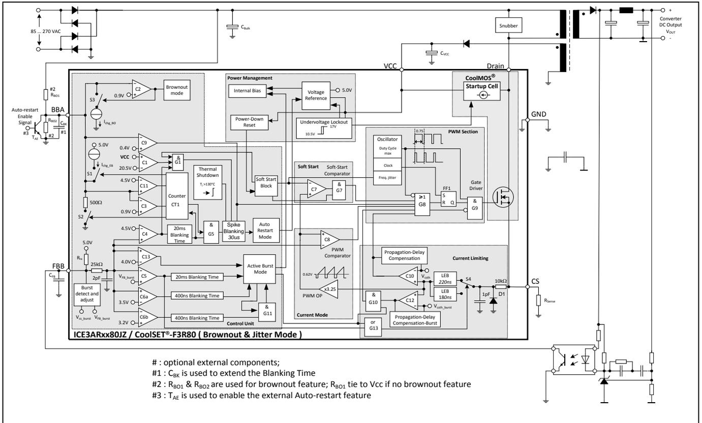
Figure 3 Representative Block Diagram
