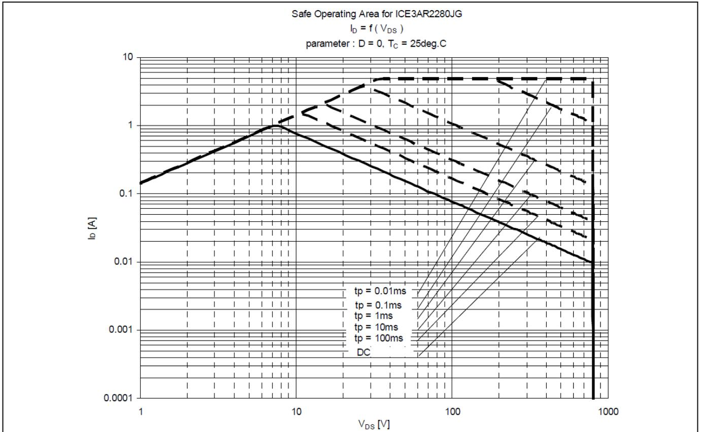
Figure 36 Safe Operating Area (SOA) curve for ICE3AR2280JG
