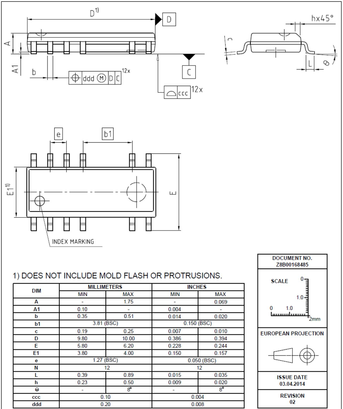
Figure 42 PG-DSO-12 (Pb-free lead plating Plastic Dual-in-Line Outline)
