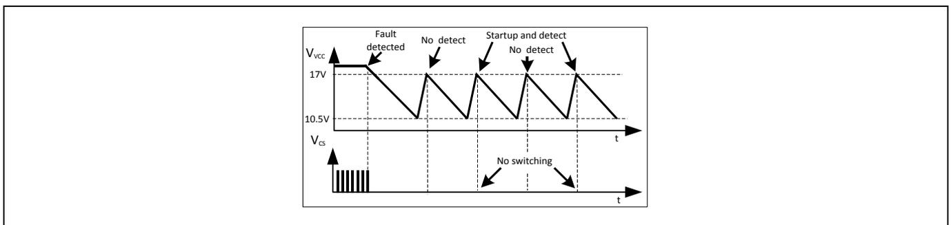
Figure 31 Odd skip non switch auto restart waveform
