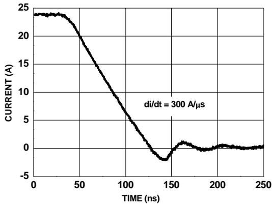
Figure 14. FDMS8025S SyncFET body diode reverse recovery characteristic
