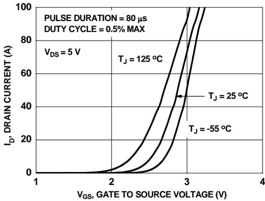
Figure 5. Transfer Characteristics
