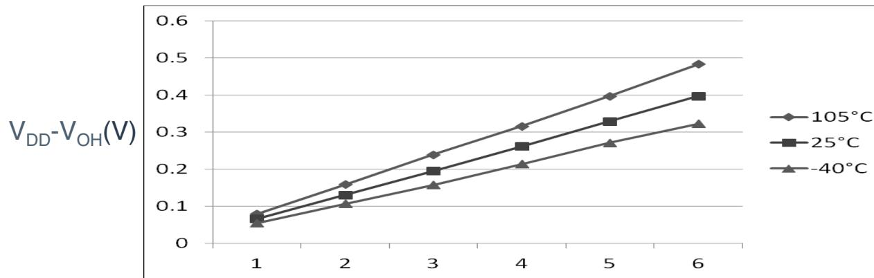
Figure 1. Typical  $V_{DD} - V_{OH}$  Vs.  $I_{OH}$  (standard drive strength) ( $V_{DD} = 5\text{ V}$ )
