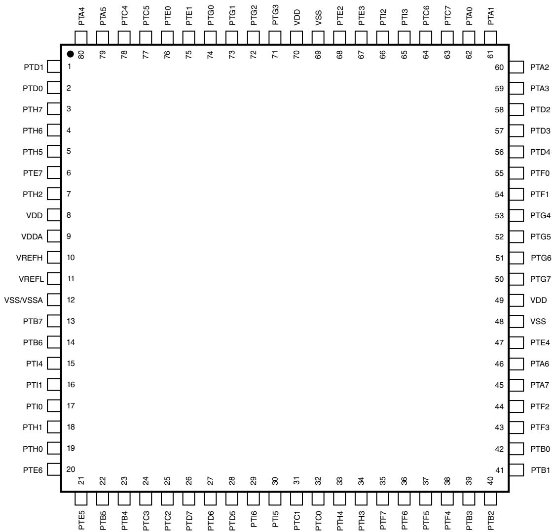
Figure 21. 80-pin LQFP package
