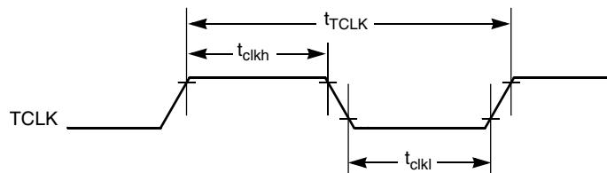
**Figure 11. Timer external clock**
