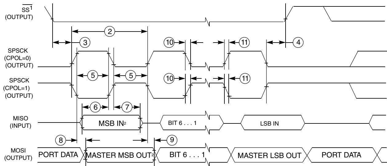
**Figure 18. SPI master mode timing (CPHA=1)****Table 18. SPI slave mode timing**
