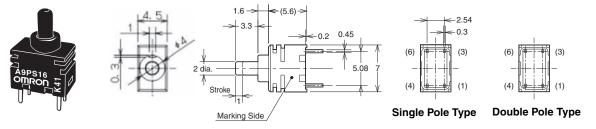
Note: NO.(4) and (6) terminals in the SPDT models are dummys to support the Switch case.
