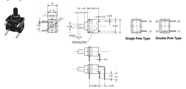
Note: Unless otherwise specified, a tolerance of  $\pm 0.4$  mm applies to all dimensions.
