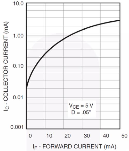
Figure 2. Normalized Collector Current vs. Forward Current
