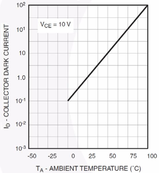
Figure 4. Normalized Collector Dark Current vs. Temperature
