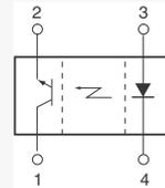
PIN 1. Collector    PIN 3. Anode
